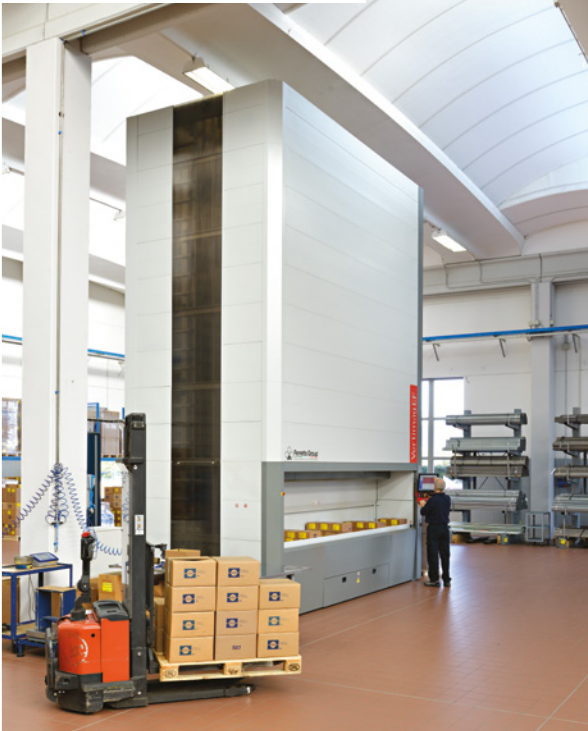
AUTOMATED SMALL PARTS WAREHOUSE
